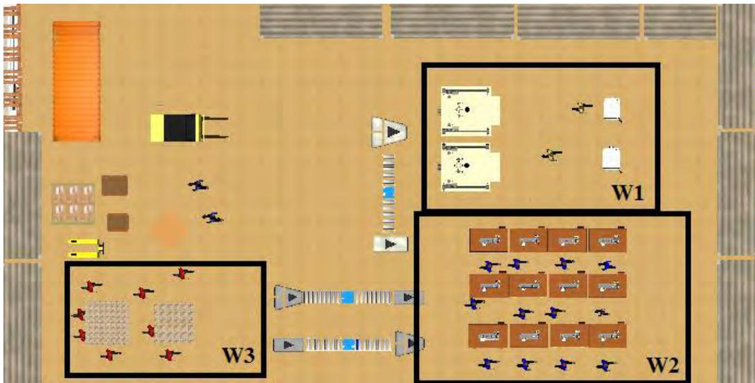
Figure 2: 2D-view of the layout designed through the simulation software (W1: Work centre 1, W2: Work centre 2 and W3: Work centre 3).
