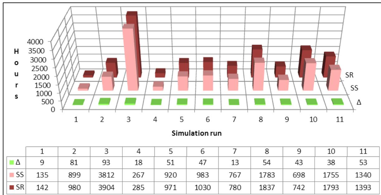
Figure 4: Simulation results expressed as the total time required in 'as is' scenario ( $S_R$ ), the total time required in the new scenario simulated ( $S_S$ ) and the time savings (in hours).
